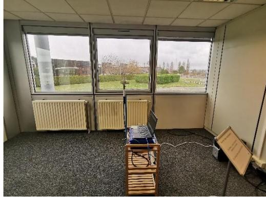
Figure 1: Frequency selective measurement system installed at a stationary position
