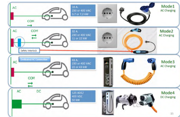
Charging modes according to standard IEC 61851-1
