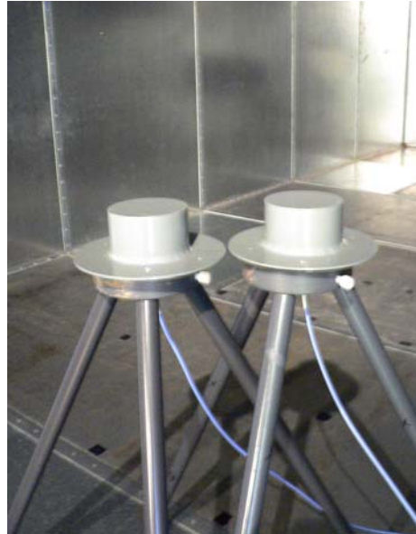
Fig. 2 Two conical monopole antennas placed inside a reverberation chamber
