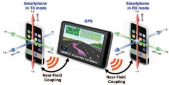
Fig.3: Near-Field coupling between two smartphones with and without interferer (*GPS device in operation*).
