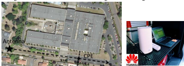
Figure 1 : on the left, satellite view of the 5G site at Bordeaux-Mérignac, position of the CPE receiving the data and axis of measurements; and on the right, CPE custom premise equipment used to receive the 5G data.
