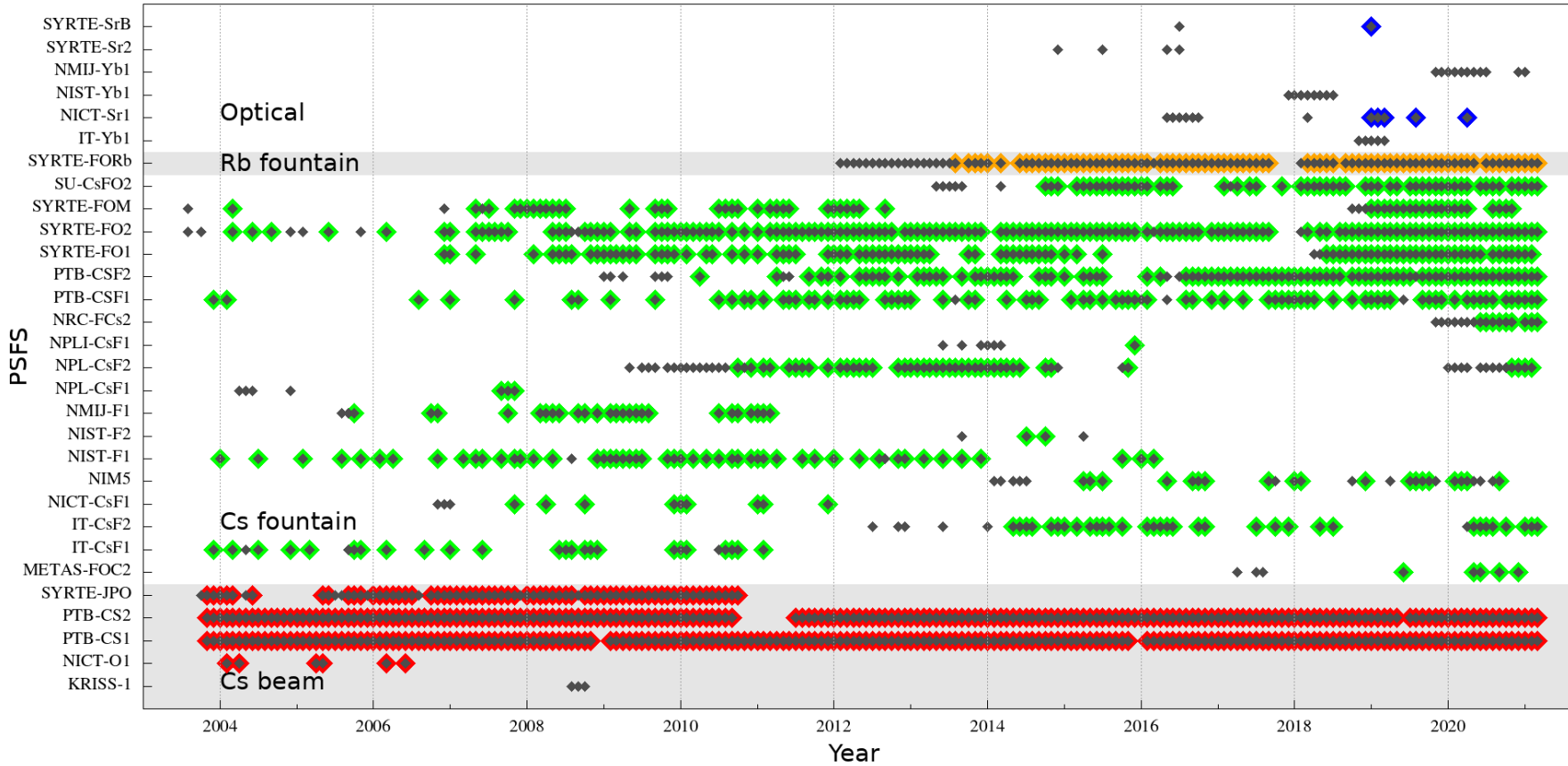
Graphical representation of all evaluations of Primary and Secondary Frequency Standards reported since Circular T 190. Enhanced color dots indicate evaluations carried out within the month of TAI computation.
